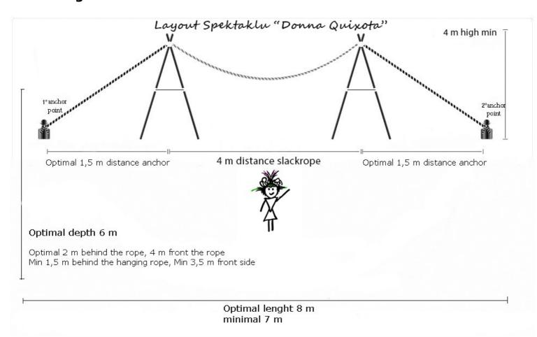
\*The anchor points for the slack wire: we need 2 x 1980 lbs/ 900 kg. In another document I enclosed the Rigging Options.
